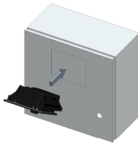
Fig. 3: Installing the control unit in the control cabinet
